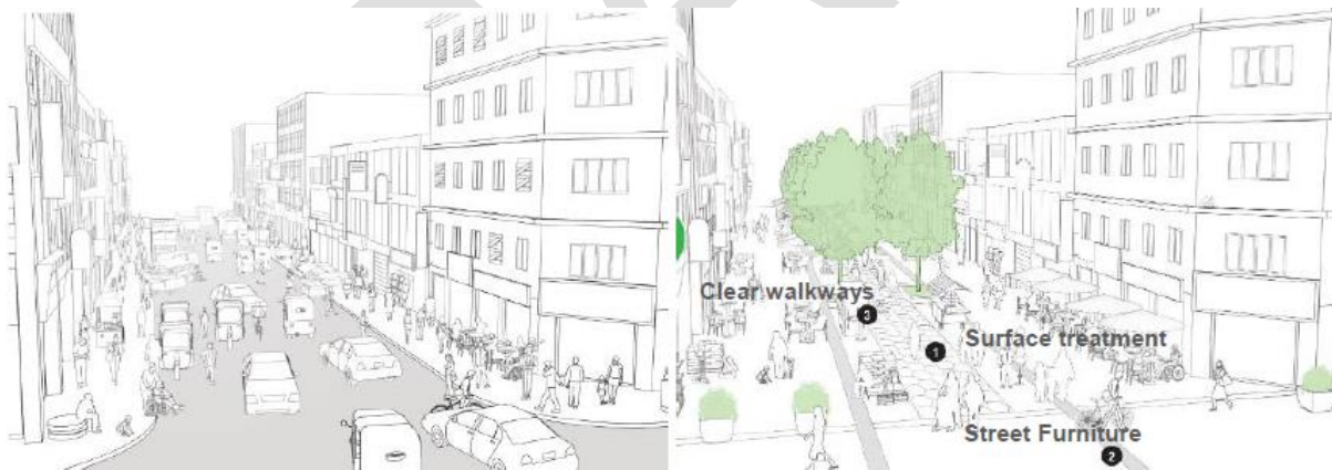
Figure 163 Representation of before and After of NMT Streets
