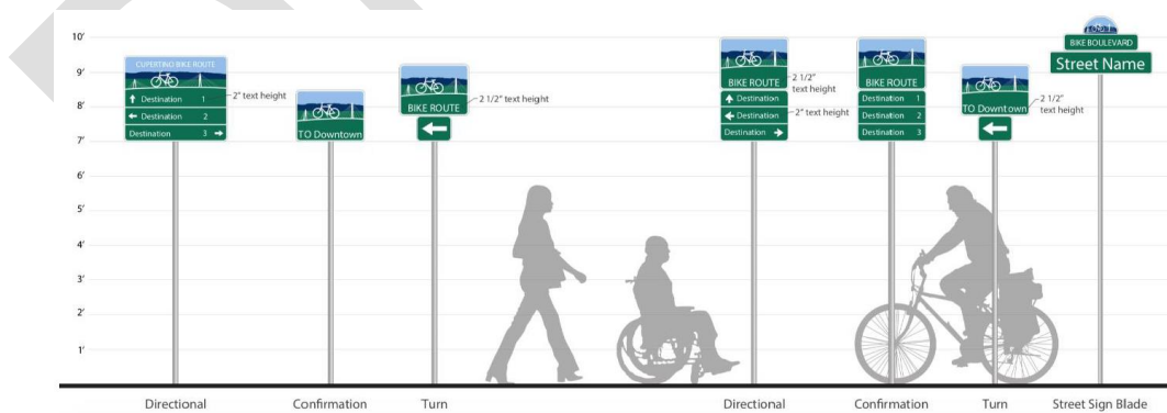
Figure 159 Representation of Wayfinding and Signage Boards Heights 10
