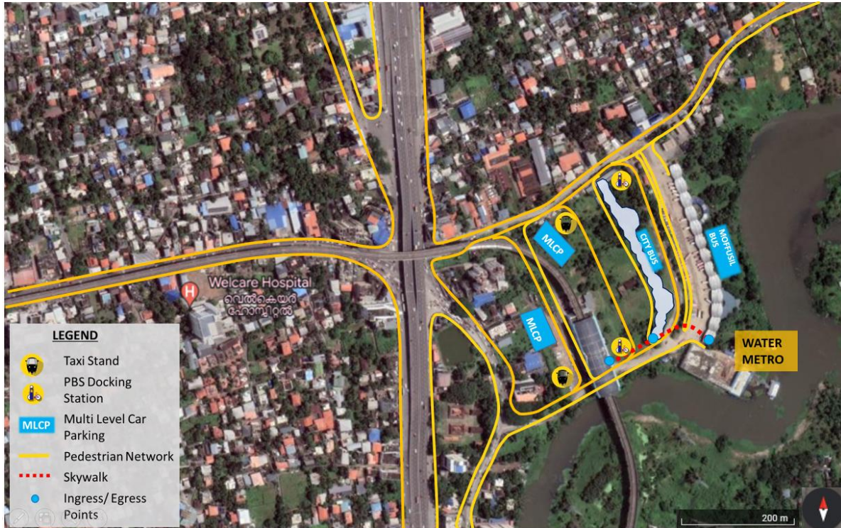
Conceptual Plan of suggested improvement measures at Vyttila Junction and Vyttila Mobility Hub
