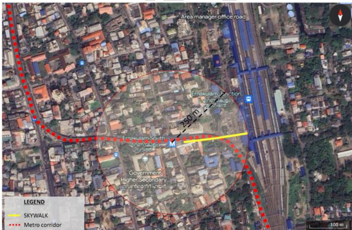
Figure 180 Skywalk Proposal for Ernakulam South Railway station from Metro Station
