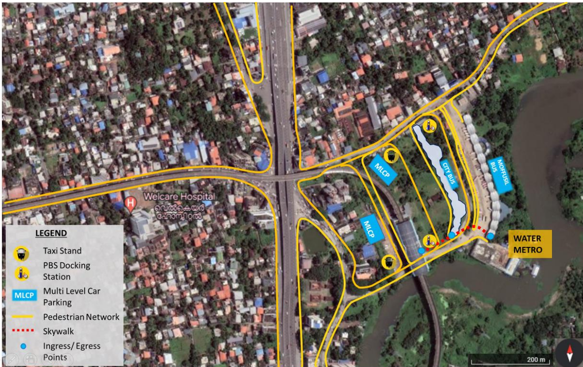
Figure 177 Conceptual Plan of suggested improvement measures at Vyttila Junction and Vyttila Mobility Hub
