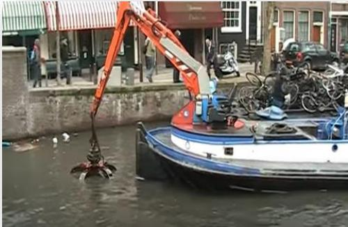
**Figure 4A.1(a) Grabbers mounted on pontoon to remove dumped solid waste**
