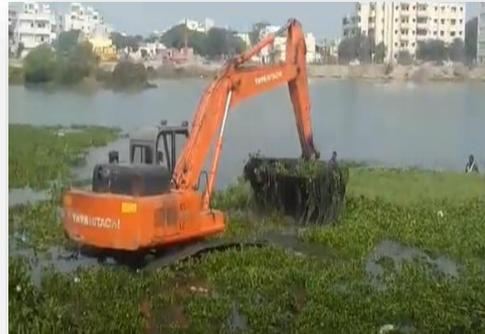
**Figure 4A.1(b) Conventional method of Hitachi mounted on pontoon**
