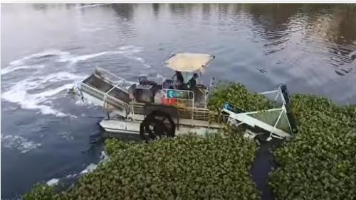
**Figure 4A.1(c) Aquatic weed harvester (cleaning process)**
