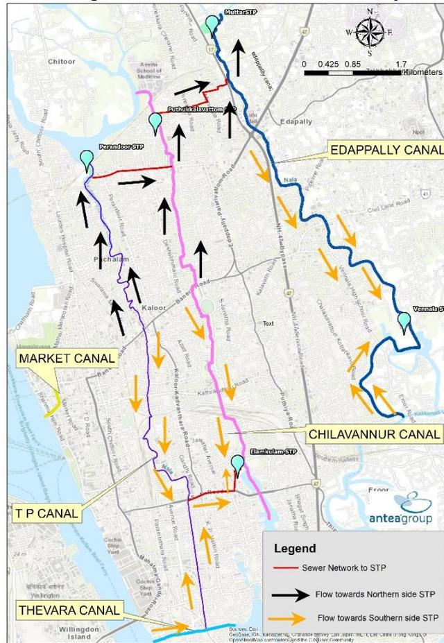
**Figure 2.15: Sewer load flow direction**
