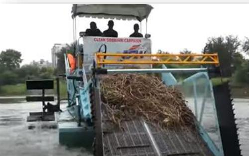
**Figure 4A.1(e) Water hyacinth the floating materials harvester with conveyor belts (Large)**
