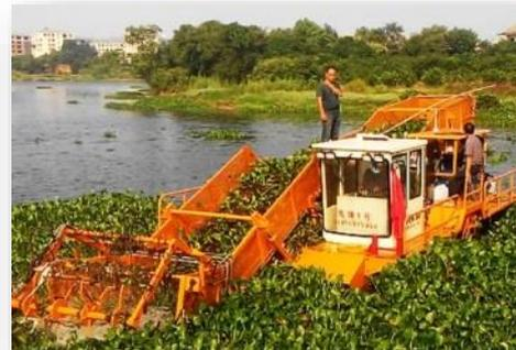
**Figure 4A.1(f) Water hyacinth the floating materials harvester with conveyor belts (Small)**
